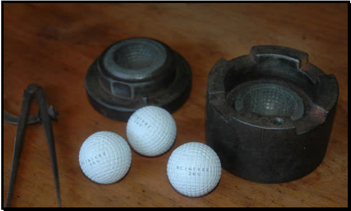
Gutta percha golf balls made from authentic 1890 line cut cast iron mold
